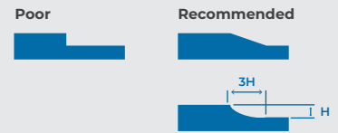
Fig. 1.2 Illustration of inside & outside draft angle to allow easy component removal fro tool.
