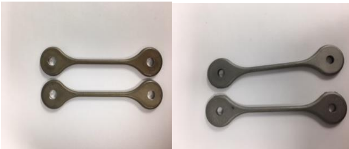
Figure 1. 17-4PH Tensile bars made by MIM (left) and Printalloy® (right)
