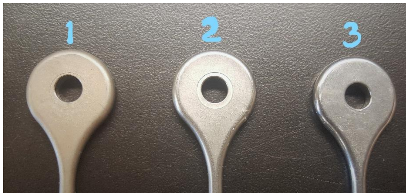
Figure 4. MIM tensile bars as a function of their surface treatment groups
